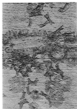
Fig. 6. Crystal growth of phosphate coating on polished pure iron (26 min). ( \times 180 )
