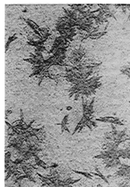
Fig. 3. Crystal growth of phosphate coating on polished carbon steel (10 min). ( \times 180 )
